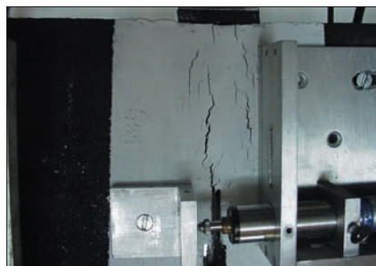
HaTelit® -reinforced specimen: bending failure after 490,000 cycles
