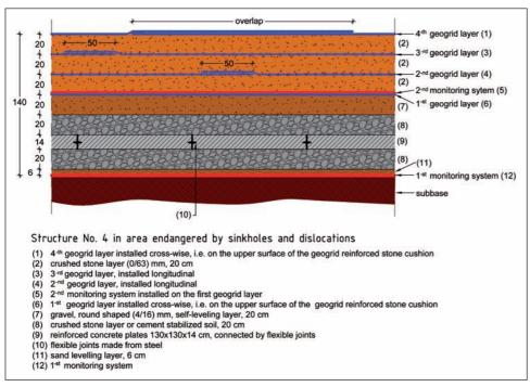
Fig. 9: Designed cross section, structure no. 4
