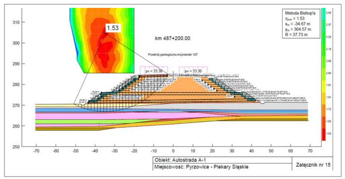
Fig. 8: Design, check of global stability of motorway embankment, Bishop's method
