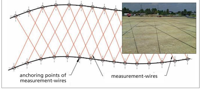
Fig. 10: 1st monitoring system (warning layers) diagonal installed measurement wires, System NeoStrain®
