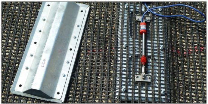
Fig. 12: 2<sup>nd</sup> Monitoring system on Fortrac<sup>®</sup> geogrid, system NeoStrain<sup>®</sup>
