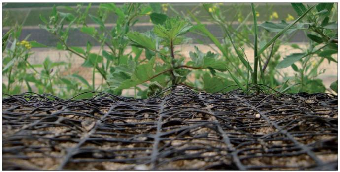
Fig. 14: Close up of Fortrac 3D<sup>®</sup> structure supporting the vegetation
