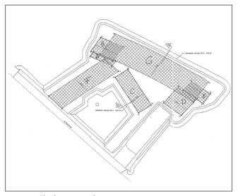
Geotextile lay-out plan
